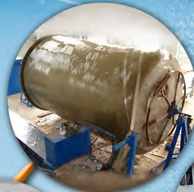
TANK FABRICATION BY FILAMENT WINDING MACHINE
